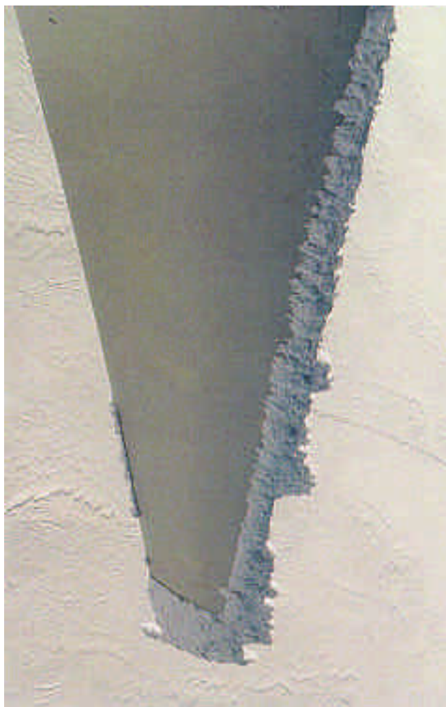
Iced leading edge of a rotor blade operating in Switzerland
