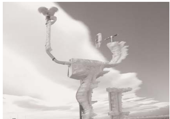
Fig. 6: EUMETNET wind sensor test at Mont Aigoual in France. Degréane DEOLIA96 sensors are currently used in the Météo-France network. This model has shaft heating. Cups on the left and the vane on the right [ 4].
