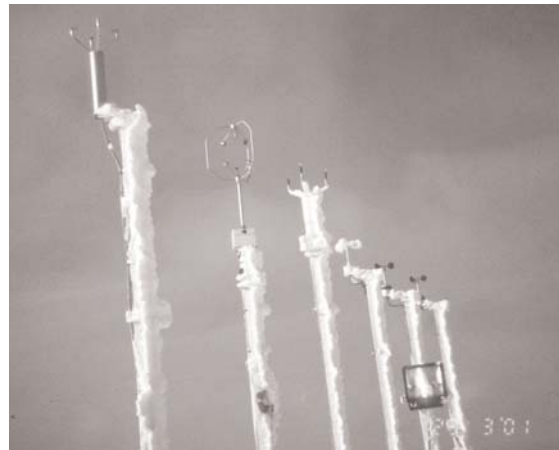
Fig. 4: EUMETNET wind sensor test at Luosto fell in Finland. Different sonic and cup anemometers under icing conditions [ 4].
