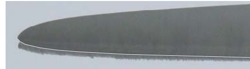
Fig. 3 Typically iced rotor blades, here examples at MW turbines. The leading edge contour is marked by the white line.
