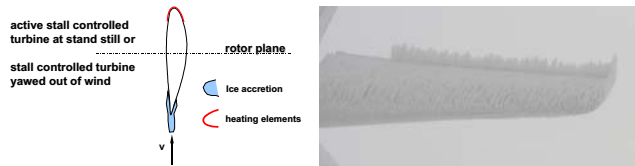
Fig. 5 Stall-controlled wind turbine in icing conditions at standstill: Possible configuration if only the leading edge is heated. Observation of trailing edge icing (right side) of a stall-controlled turbine at stand still.
