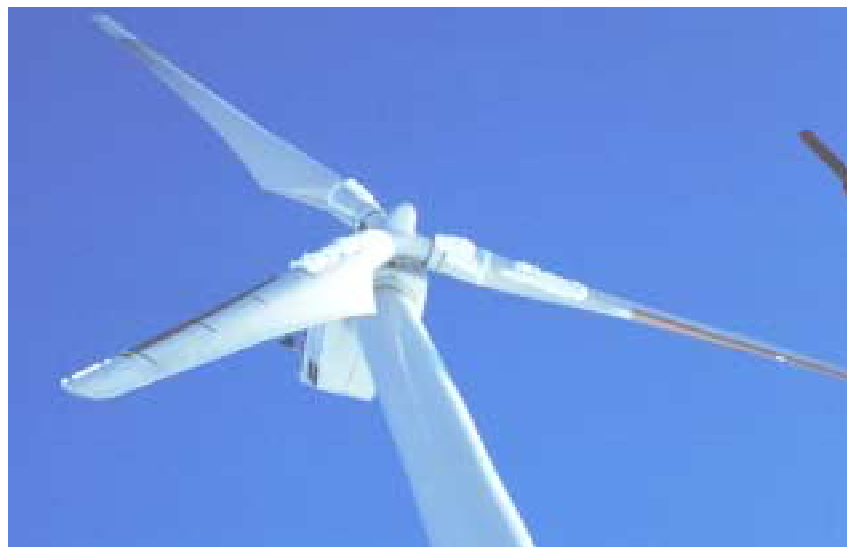
Figure 11 Wind turbine suited for icing conditions: Heating elements at the leading edge.
