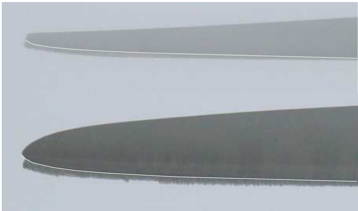
Figure 6 Typically iced rotor blades, here examples at MW turbines. The leading edge contour is marked by the white line.
