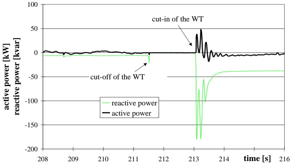
Fig. 3: Cut-off and cut-in of the generator of the WT.
