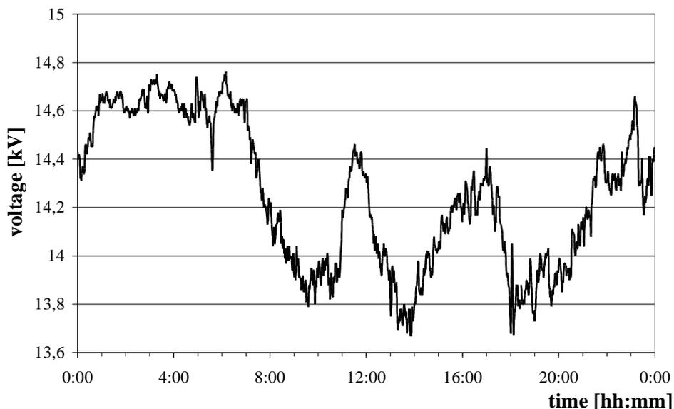
Fig. 4: Voltage changes on 23. Sept. 1997 at the medium voltage grid of the wind farm
