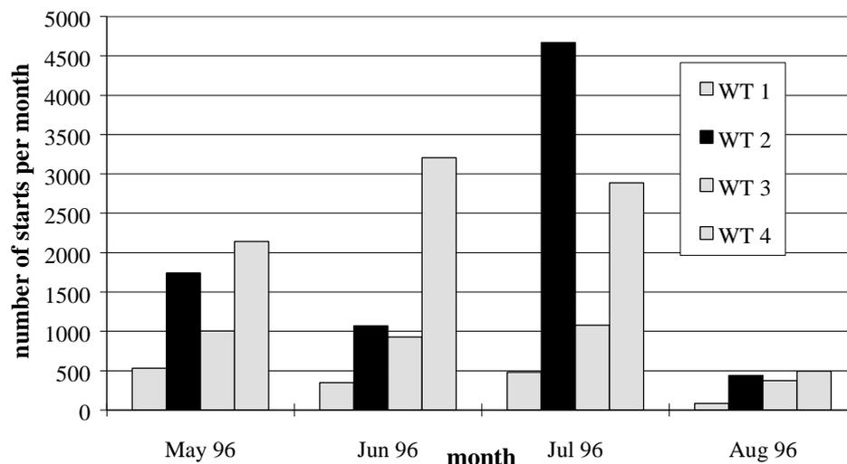
Fig. 1: Number of starting operations per month for each turbine.
