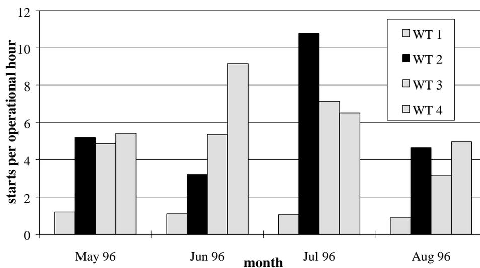
Fig. 2: Number of starting operations per operational hour for each wind turbine.
