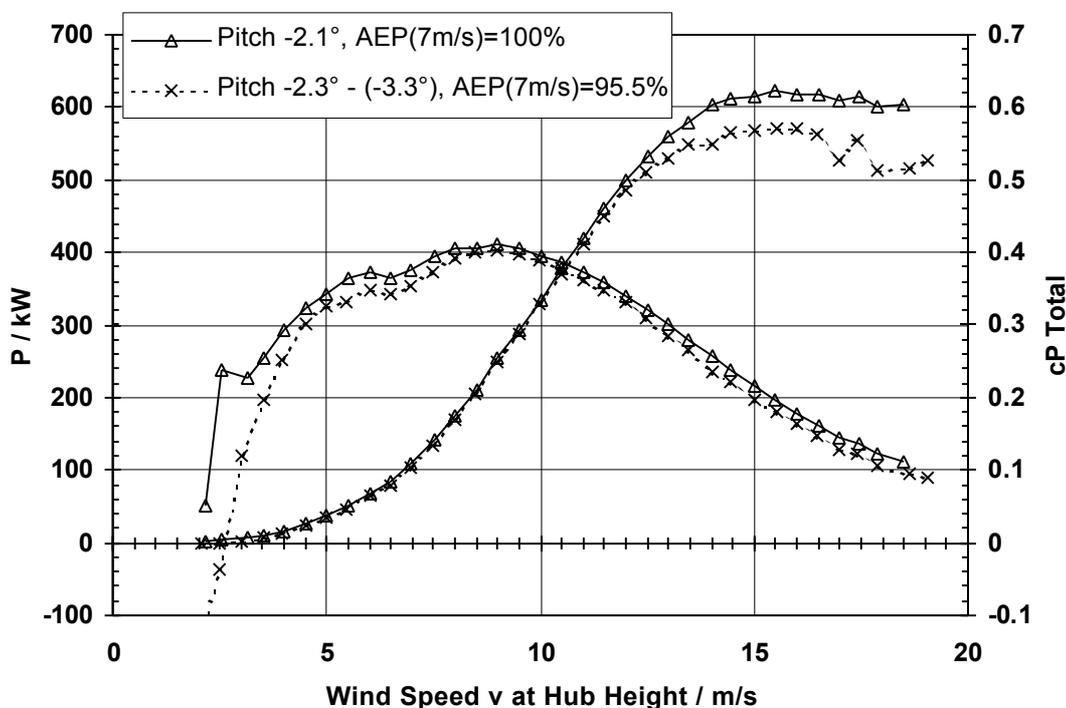
Fig. 1: Power curves of a stall regulated WTGS for different pitch settings. A small imbalance between the pitch angles of different rotor blades of about  $1^\circ$  leads to a decrease of about 5% in the annual energy production.
