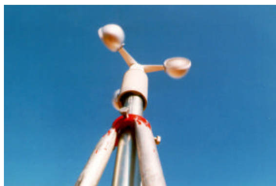
Fig. 3: Left picture: best practice of anemometer mounting (mast lying on the ground before the erection); the anemometer is positioned on a long pole exceeding the mast. The lightning receptor as well as the vane are mounted far away from the anemometer. Right picture: poor practice of anemometer mounting, the anemometer on the right picture is mounted too close to the mast structure and is not aligned absolutely vertically.
