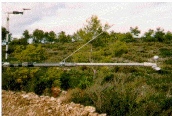
Fig. 3: Left picture: best practice of anemometer mounting (mast lying on the ground before the erection); the anemometer is positioned on a long pole exceeding the mast. The lightning receptor as well as the vane are mounted far away from the anemometer. Right picture: poor practice of anemometer mounting, the anemometer on the right picture is mounted too close to the mast structure and is not aligned absolutely vertically.
