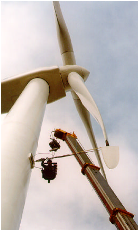
Fig. 2: Calibration of the blade root bending moment in flapwise direction.
