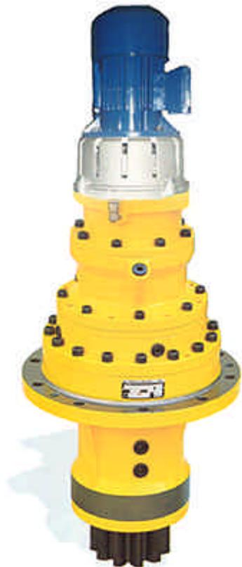
Fig. 3: A soft yaw drive with a yaw gearbox, a hydrodynamic coupling in an enclosure and an electrical motor with a brake.
