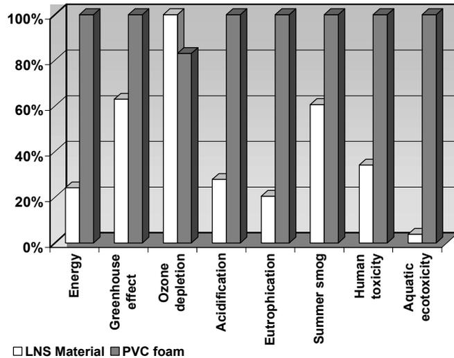
Fig. 5: Environmental profiles of LNS and PVC foam.
