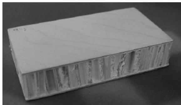
Fig. 1: The principal structure of LNS and manufactured test specimen.
