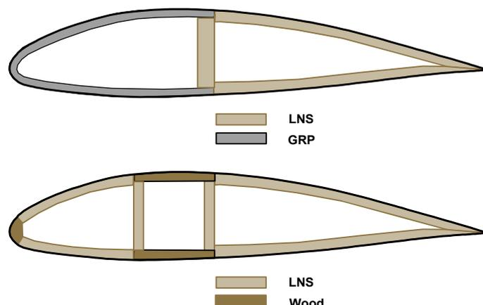
Fig. 4: Two examples of the rotor blade cross section which have been investigated in the design study.
