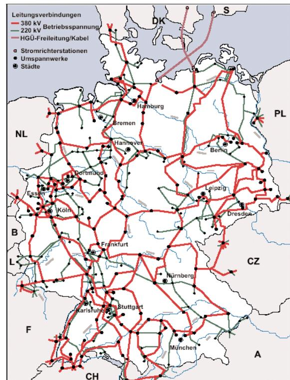
Fig. 4 High voltage distribution grid of E.on. Circles indicate the possible grid feed-in points in northern Germany [2]
