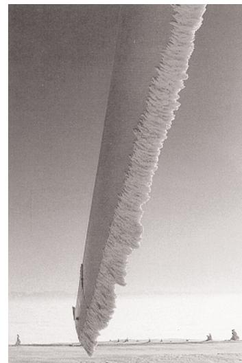
Fig. 5: Iced wind turbine blades in Germany.
