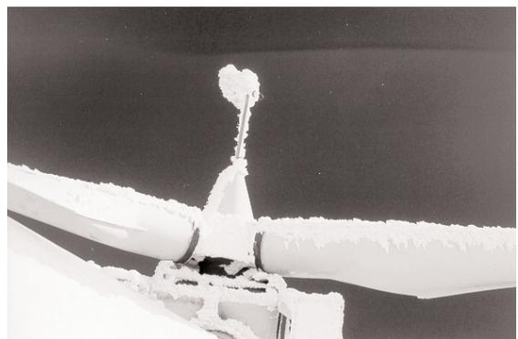
Fig. 7: Iced blades and control anemometer in Switzerland.
