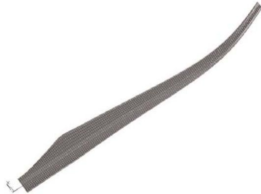
Fig. 2: Third normal mode of the blade
