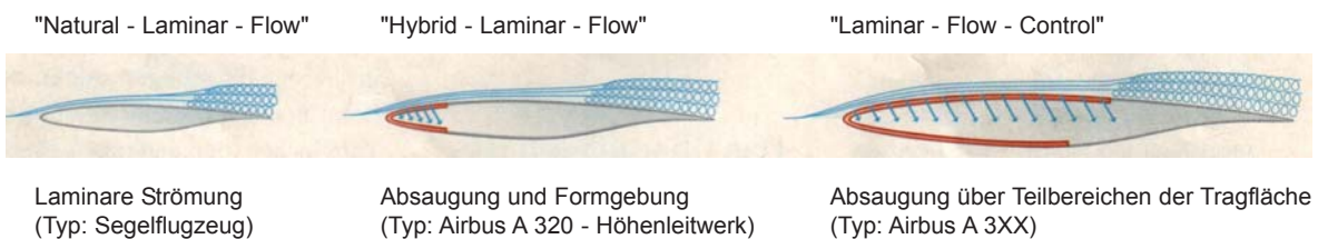
Abb. 1: Verschiedene Methoden der Grenzschichtabsaugung Fig. 1: Several methods of "boundary layer suction"
