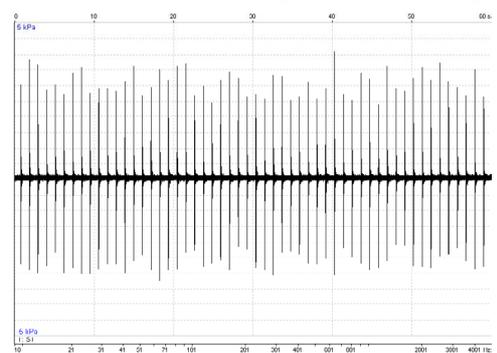
Fig. 5: 60 seconds plot of pile driving (sound pressure)
