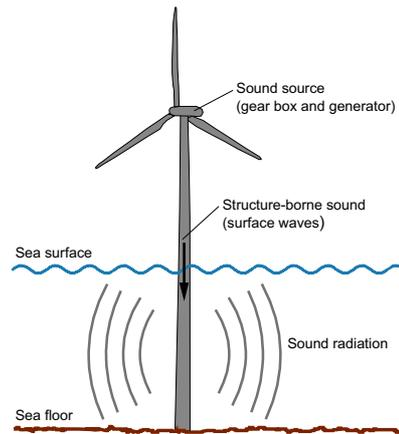
Fig. 2: Acoustic noise from operating offshore wind turbines
