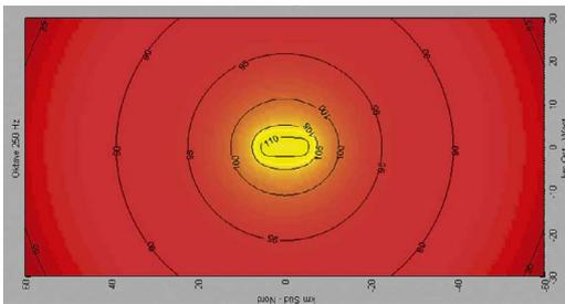
Fig. 3: Example: Prognosis of underwater sound pressure levels of a hypothetical wind farm of 70 turbines for the 250 Hz octave band
