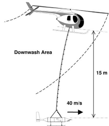
Fig. 1: The principle of the Helipod-flight: At a true airspeed of 40 ms<sup>-1</sup> the system is out of the downwash area.
