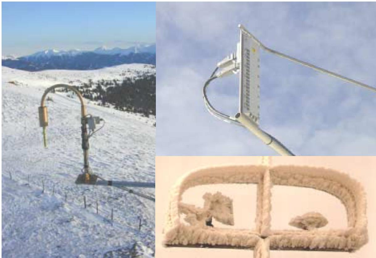
Figure 3 Direct and indirect ice sensors
