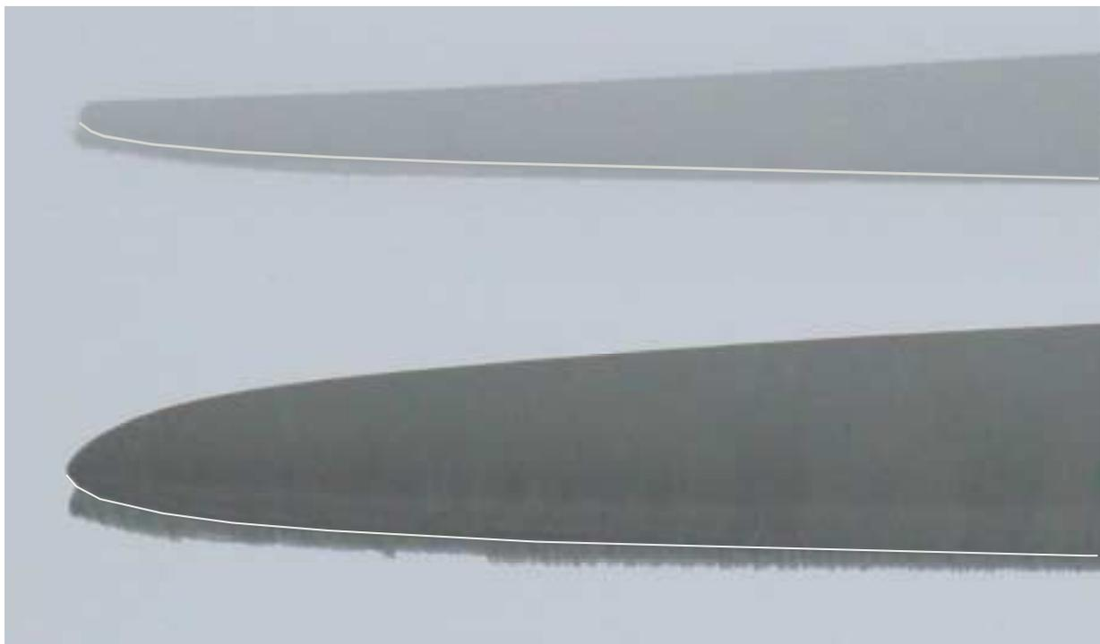
**Figure 6** Typically iced rotor blades, here examples at MW turbines. The leading edge contour is marked by the white line.
