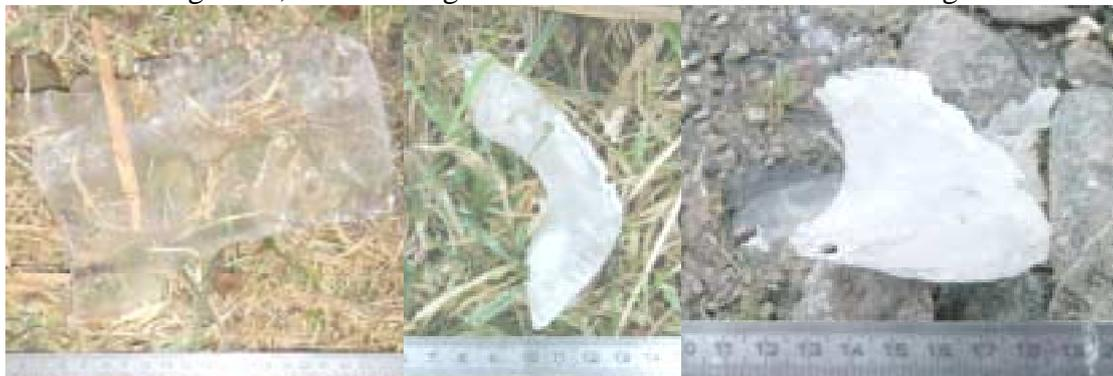
**Figure 2** Typical ice fragments taken from rotor blades or found on the ground. From the left: Glace ice origin from the rotor of a MW turbine, glace and rime ice from a 500 kW turbine.
