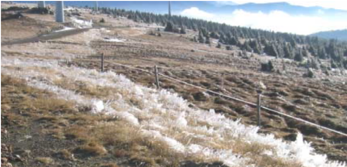
Figure 1 Nice view, but the rime ice accretion on the grass and the fence signalises danger of ice throw in the neighbourhood of the wind turbines.
