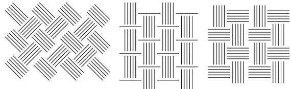
Fig. 5: Different type of textures of fiber reinforcement plastic.
