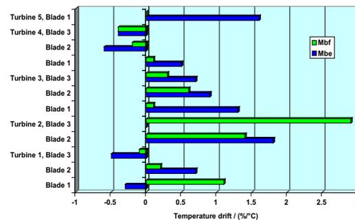
Fig. 2: Temperature drift of edgewise Mbe and flatwise Mbf bending moment (between start up and rated wind speed) related to the dead mass calibration cycle.
