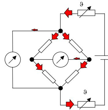
Fig. 8: Six wire bridge connections measure the voltage relation between the two arms of a Wheatstone bridge without influence of bridge supply cable.
