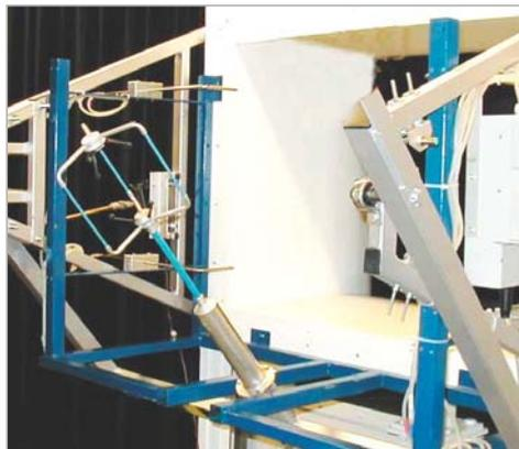
3D Calibration of sonic anemometers
