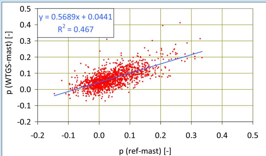
Fig. 2: Wind shear exponent  $p$  at WTGS-mast versus  $p$  at ref-mast (sc 1) for expected later measurement sector, wind speed range: [4 m/s ; 16 m/s], temperature > 2°C.
