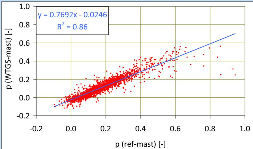
Fig. 1: Wind shear exponent  $p$  at WTGS-mast versus  $p$  at ref-mast (sc 4) for expected later measurement sector, wind speed range: [4 m/s ; 16 m/s], temperature > 2°C.
