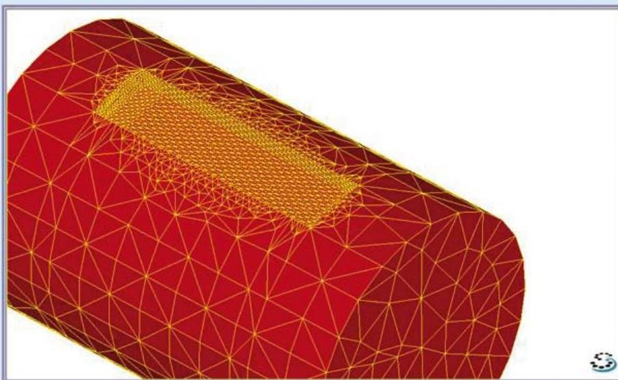
Fig. 7: Mesh on the shaft and on the keyway
