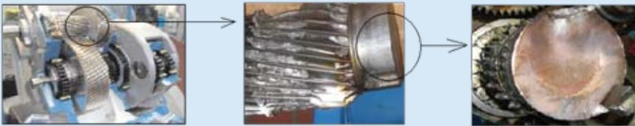
Fig. 2: The broken shaft at the middle stage of the gearbox of a wind turbine
