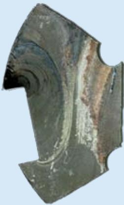
Fig. 3: Section of the shaft where failure occurred
