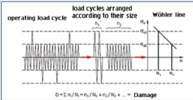
Fig. 1: Classification of load cycles according to Miner
