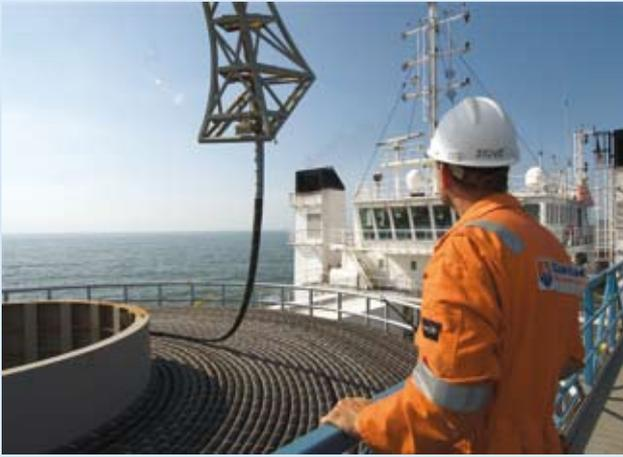
Fig. 2: Turntables on the "Team Oman" ship with 55 kilometers of cable
