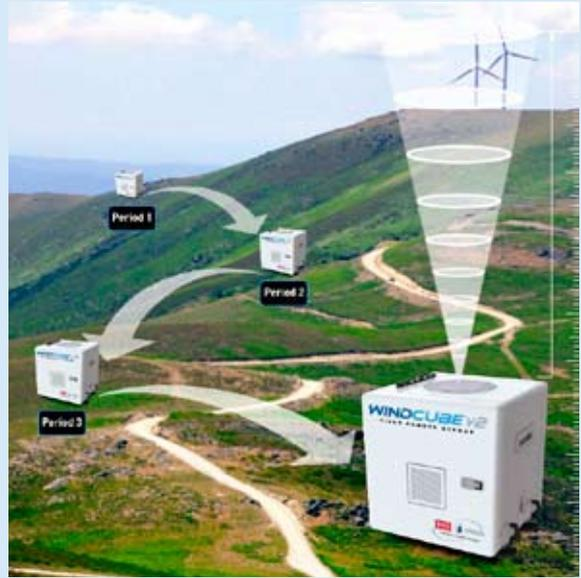
Fig. 3 : Optimised wind measurement strategy using a Lidar moved onto several locations to reduce uncertainties related to both horizontal and vertical wind speed extrapolations.
