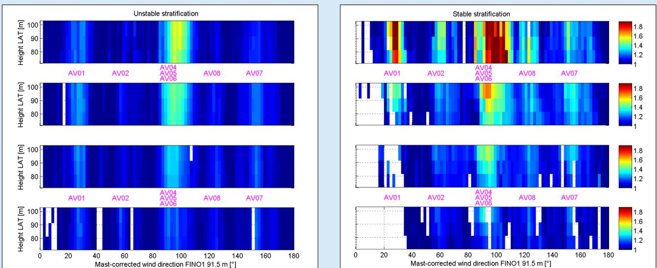
Fig. 5: Park correction factor for different heights shown in color above wind direction for 4 different wind speed bins (as in Fig. 4) for unstable stratification in the left-hand graph and for stable stratification in the right-hand graph.
