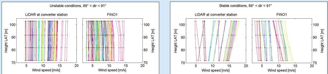
Fig. 3: Wind speed profiles measured during different atmospheric stabilities upstream (LiDAR) and downstream (FINO1) of alpha ventus at common heights. Same colors relate to same times of measurement.
