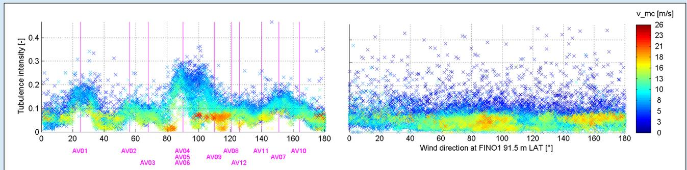
Fig. 2: In the left-hand graph (May 2011 to September 2012) the influence of alpha ventus becomes obvious in turbulence intensity depending on the wind speed depicted in color. Local maxima are related to wind turbines. In the right-hand graph (2008) turbulence intensity was evenly distributed over eastern wind directions.
