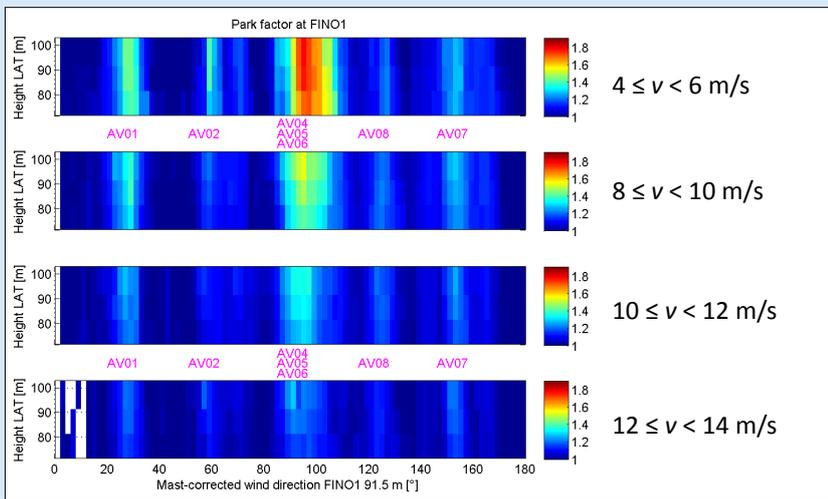
Fig. 4: Average park correction factor between 2 heights shown in color above wind direction for 4 different wind speed bins.
