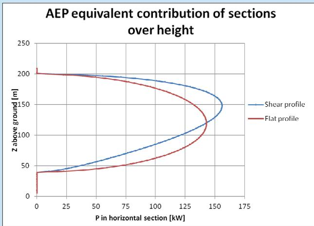
Fig. 1: Power in horizontal stripes of 2 meters height for a turbine with 120 m hub height, 160 m rotor diameter,  $\alpha=+0.25$ , 9.0 m/s wind speed at hub height. The impact of shear onto the net power in the rotor plane is a function of hub height and rotor diameter.
