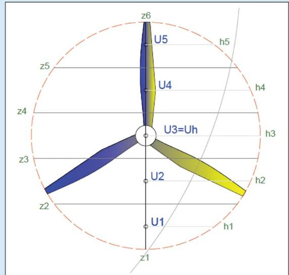
Fig. 1: Rotor area divided into five segments  $A_i$  to determine  $U_{REWS}$
